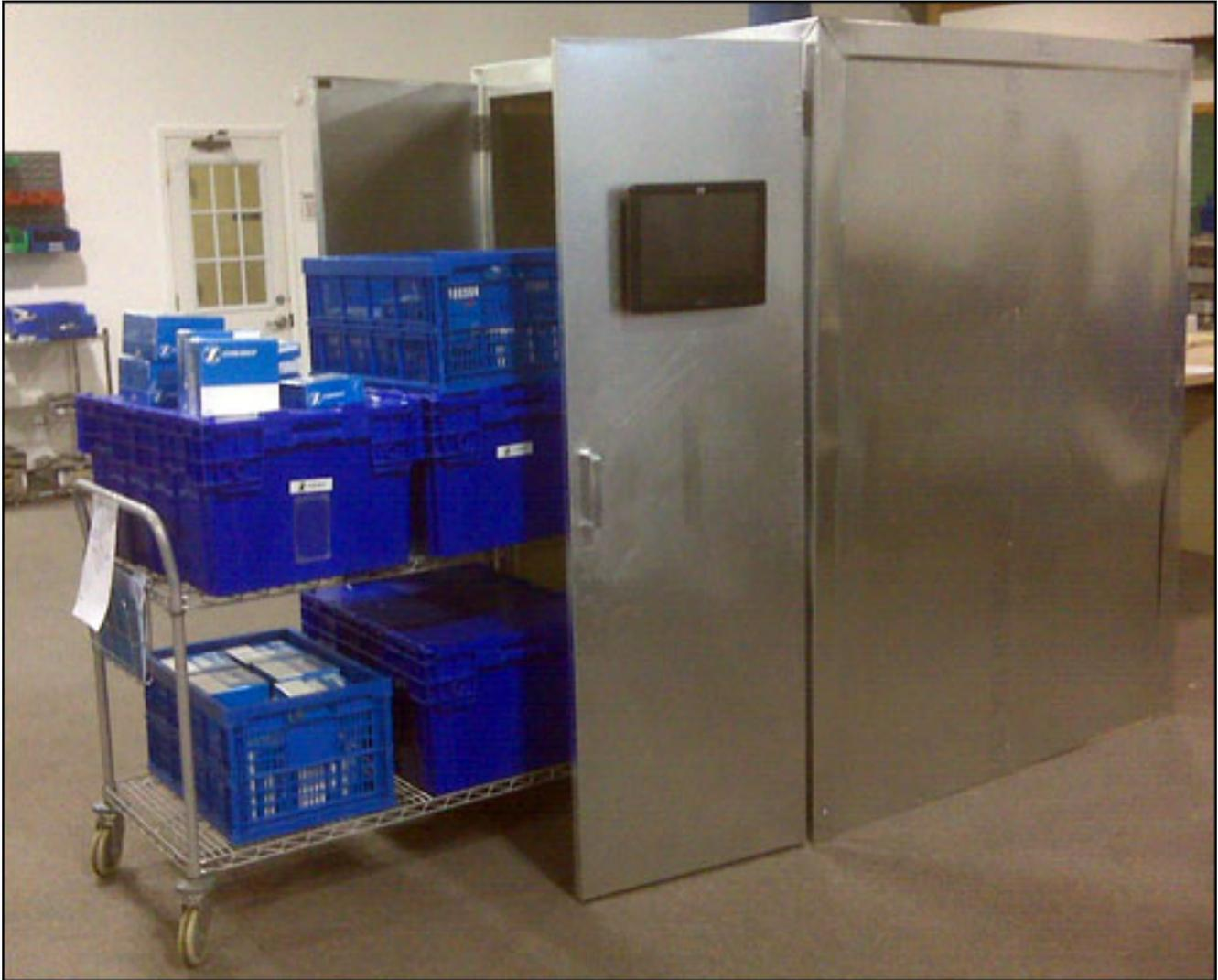
*A cart loaded with the trays and implantable devices is rolled into a custom-designed RFID tunnel.*
